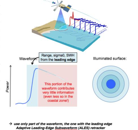
→ use only part of the waveform, the one with the leading edge Adaptive Leading-Edge Subwaveform (ALES) retracker
